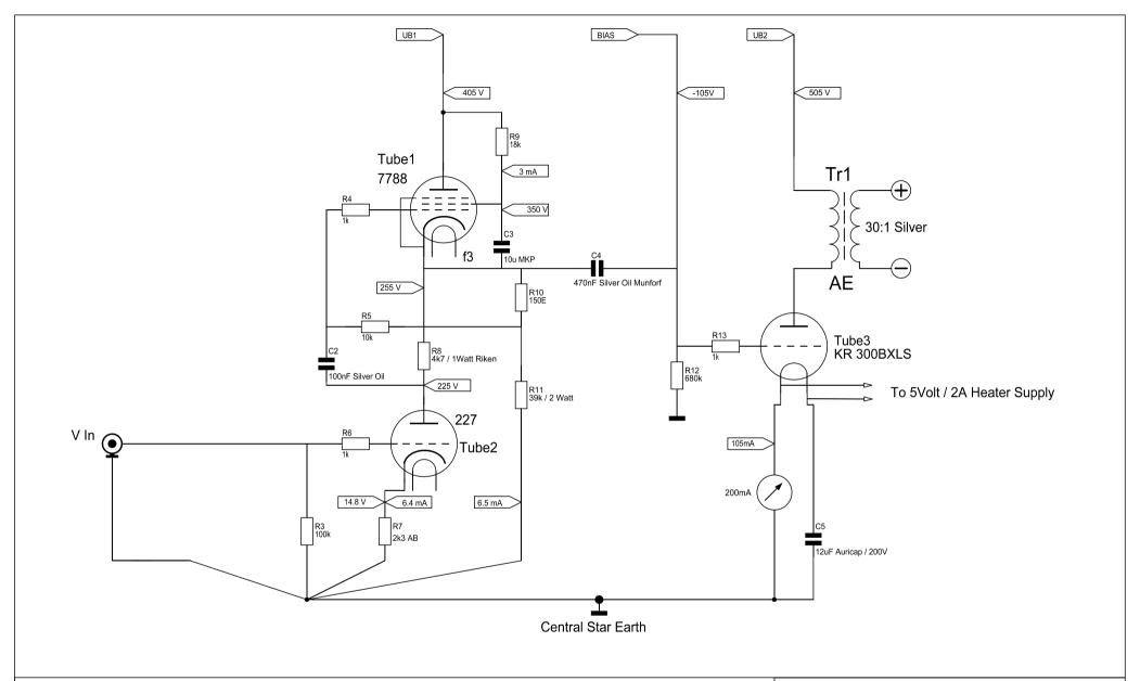
Right Channel identical to Left Channel. All parts x 2 All Resistors Carbon types unless mentioned otherwise
